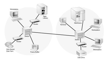
Figure 2-9. SAN with fabric configuration example
